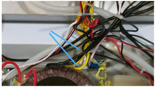
Remove connector indicated on control board.
