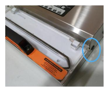
The large valve controlling sealing and releasing may need to be replaced
