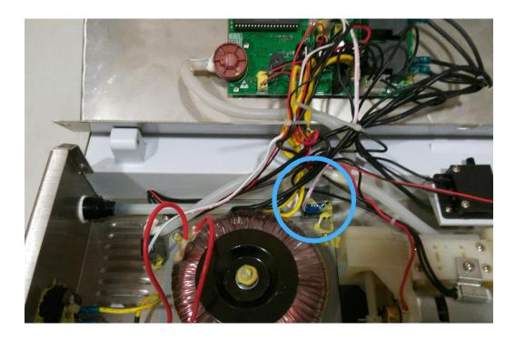
If the large valve needs to be replaced remove hoses indicated below
