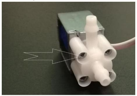
Wipe down / clean and then lubricate with CRC or WD40: (Don't use silicon spray it may swell the seals)
