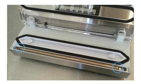
If broken, there is a replacement element shipped with the machine. Unscrew at both ends and replace.
