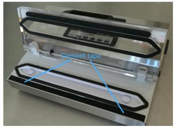
Check there are no crinkles in the black tape that covers the element, if possible flatten out the tape or replace. A spare tape is included with all machines purchased.
